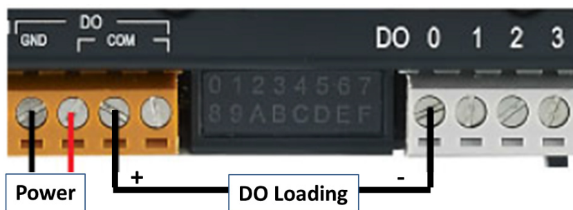
Figure 3.4 Digital Output Wiring
