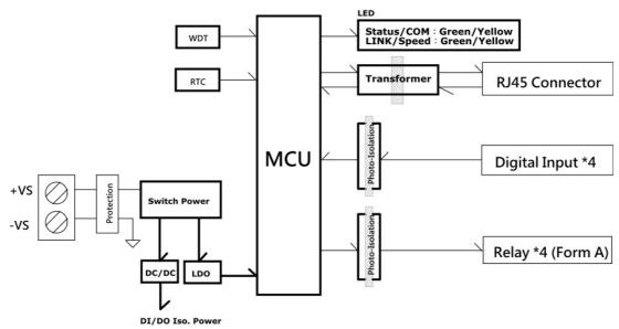
Figure 2.12 WISE-4060/LAN Block Diagram
