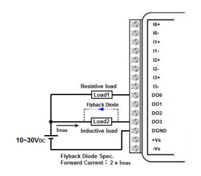
Figure 2.2 WISE-4010/LAN Digital Output Wiring Diagram
