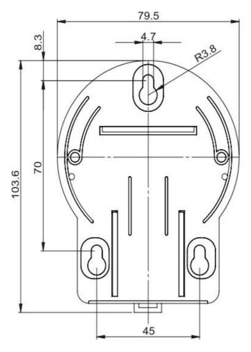
**Figure 3.5 Mounting Kit Dimensions**
