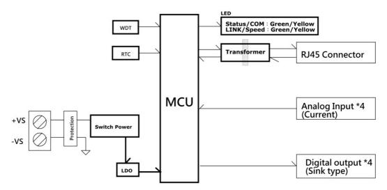
Figure 2.4 WISE-4010/LAN Block Diagram
