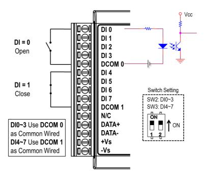
Figure 2.27 WISE-4051 Digital Input Dry Contact Wiring Diagram
