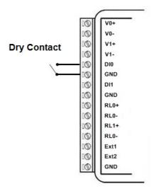
Figure 2.14 WISE-4012E Digital Input Wiring Diagram
