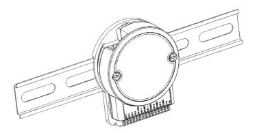
Figure 3.3 Mounting on the DIN-Rail
