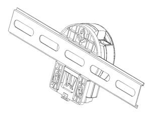
Figure 3.4 Rear View of DIN-Rail Mounting
