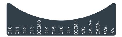
Figure 2.30 WISE-4051 Pin Assignment
