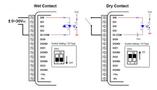
Figure 2.23 WISE-4050 Digital Input Wiring Diagram
