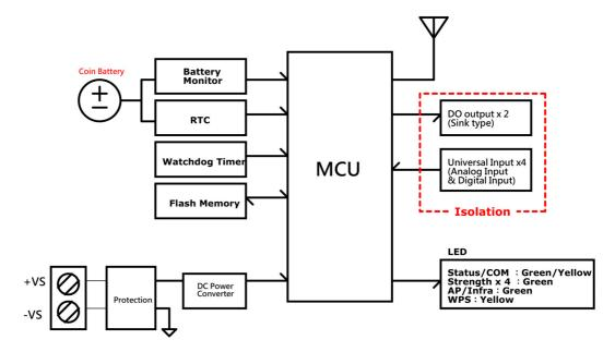
Figure 2.22 WISE-4012 Block Diagram
