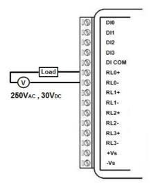
Figure 2.10 WISE-4060/LAN Relay Output Wiring Diagram
