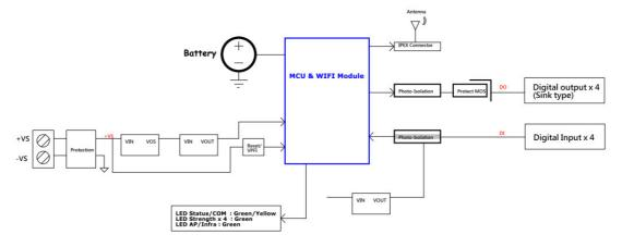
Figure 2.26 WISE-4050 Block Diagram
