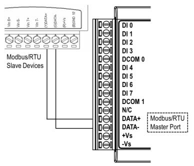
Figure 2.29 RS-485 Port Wiring Diagram
