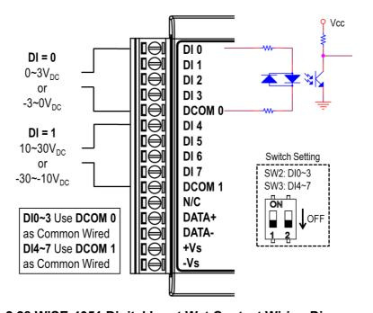
Figure 2.28 WISE-4051 Digital Input Wet Contact Wiring Diagram
