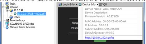
7. The "QR" tab will generate the QR code of the web configuration web page for mobile device to access the module. User can also click the QR code to open the browser for further configuration.
