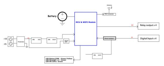
Figure 2.35 WISE-4060 Block Diagram
