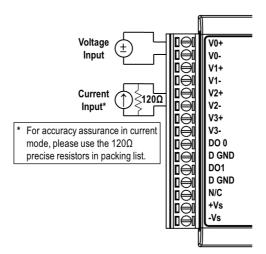
Figure 2.18 WISE-4012 Analog Input Wiring Diagram
