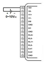
Figure 2.13 WISE-4012E Voltage Input Wiring Diagram
