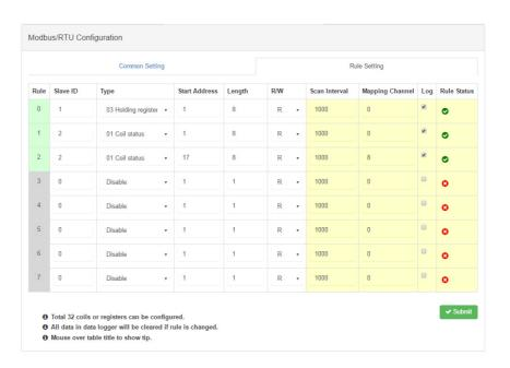
In previous figure we demonstrate how to configure an ADAM-4017+ (or ADAM-4117) which slave ID is 1 and an ADAM-4055 which slave ID is 2 as the Modbus slave devices connected to WISE-4051.
