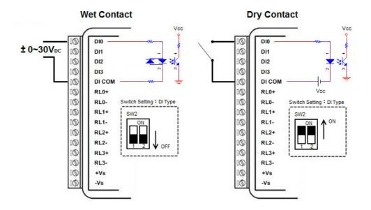
Figure 2.32 WISE-4060 Digital Input Wiring Diagram
