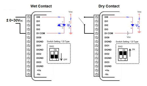
Figure 2.5 WISE-4050/LAN Digital Input Wiring Diagram
