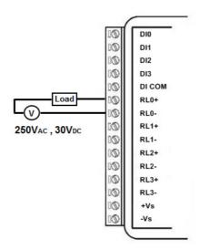
Figure 2.33 WISE-4060 Relay Output Wiring Diagram
