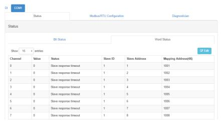
For the writable bit or word, you can click "Edit" button to switch to edit mode, change value and click "Apply" to write the Modbus address individually.
