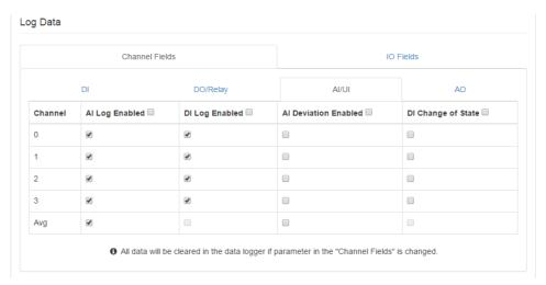
The **IO** Fields tab is to decide which Al data will be logged. Note that the log memory will be cleared once any parameter changed in the **Channel Fields** and **IO** Fields tabs.
