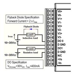
Figure 2.20 WISE-4012 Digital Output Wiring Diagram
