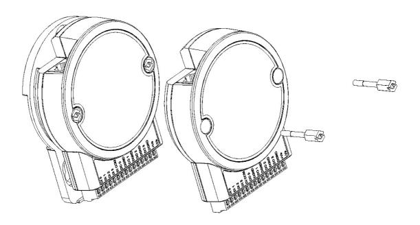
Figure 3.8 Stack Mounting
