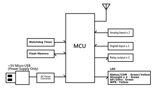
Figure 2.17 WISE-4012E Block Diagram
