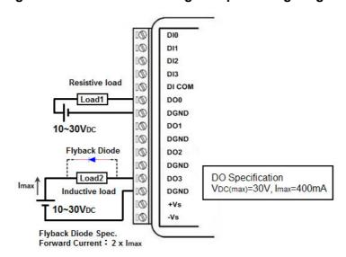
Figure 2.6 WISE-4050/LAN Digital Output Wiring Diagram
