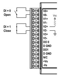
Figure 2.19 WISE-4012 Digital Input Wiring Diagram
