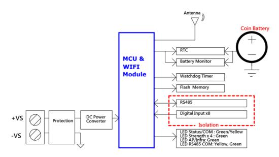
Figure 2.31 WISE-4051 Block Diagram
