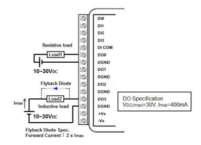
Figure 2.24 WISE-4050 Digital Output Wiring Diagram
