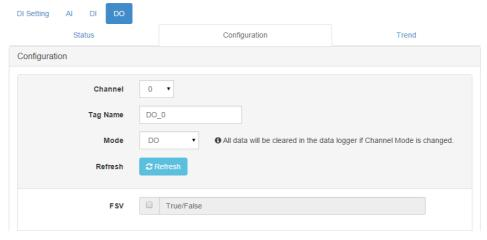
To decide whether to enable the FSV function triggered by communication with the WDT, go to **General Configuration** and enable the FSV function for all the module's output channels.
