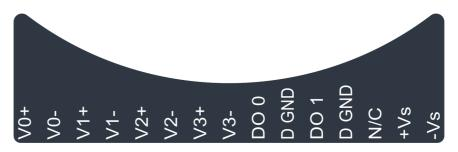
Figure 2.21 WISE-4012 Pin Assignment
