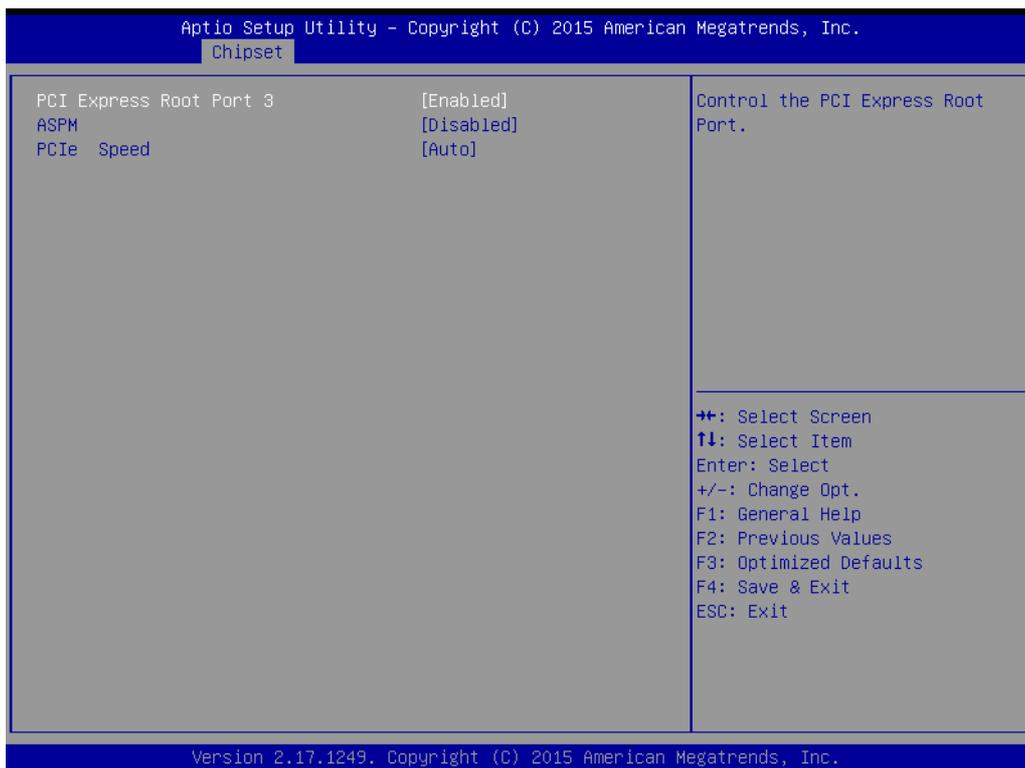
**Figure 3.38 PCI Express Root Port 3 Configuration**
