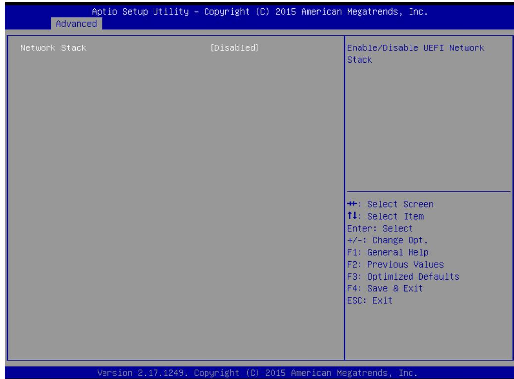
**Figure 3.23 Network Stack Configuration**
