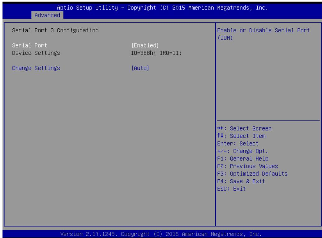
**Figure 3.13 Serial Port 3 Configuration**
