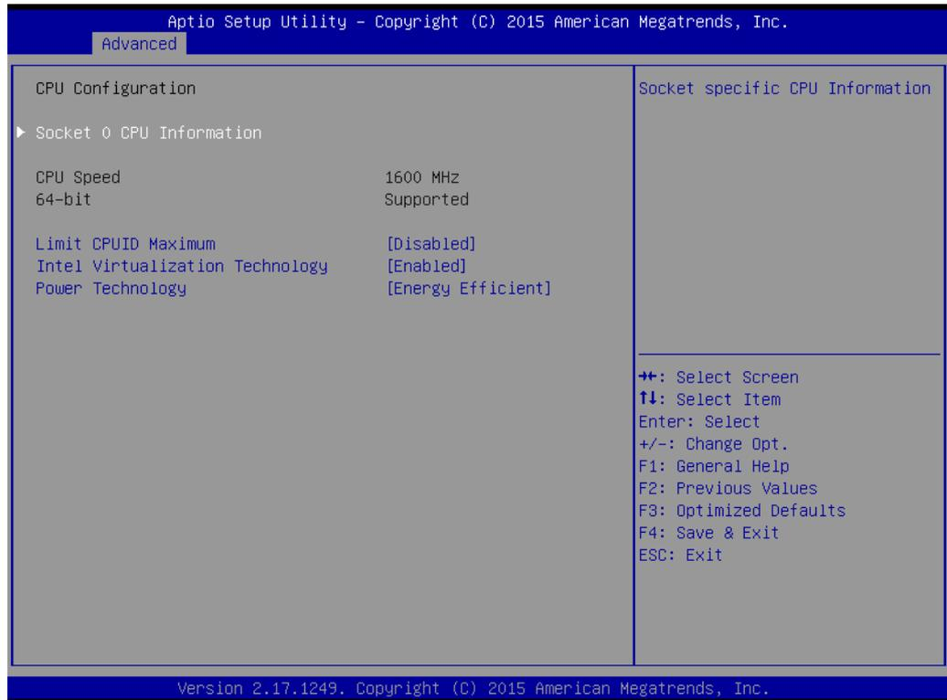
**Figure 3.17 CPU Configuration**
