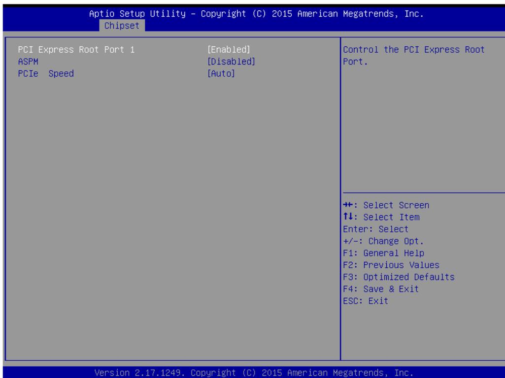
**Figure 3.36 PCI Express Root Port 1 Configuration**
