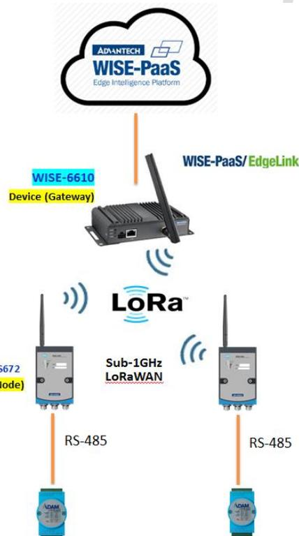
**Topology.** WISE-4610 data upload to WISE-PaaS/SCADA via Edgelinek on WISE-6610
