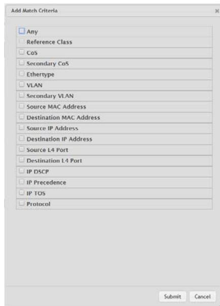
**Figure 4.405 QoS > Diffserv > Class Configuration > Add Match Criteria**
