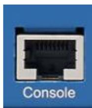
*Figure 70: RJ45 Console connector*
