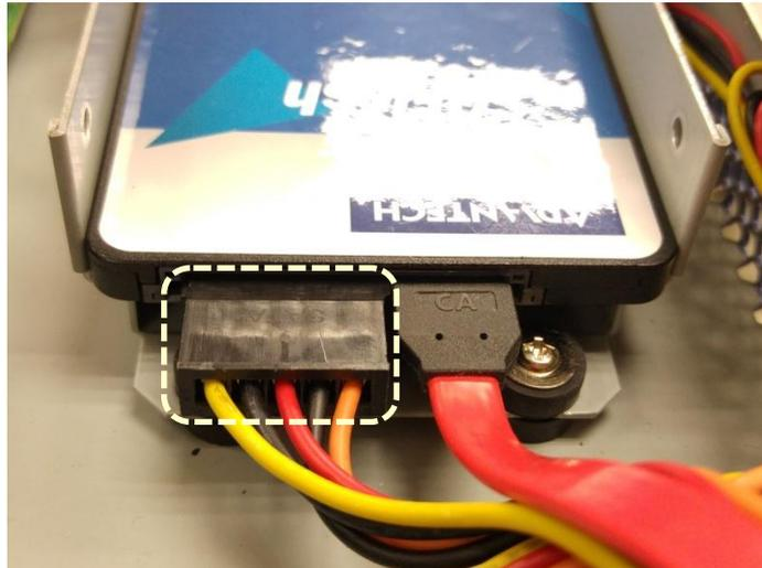
**Figure 58: HDD Power cable**
