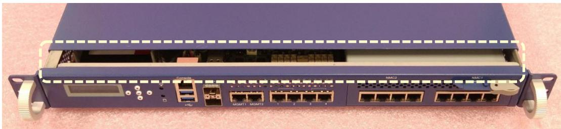
**Figure 49: Top Cover Flange Disengagement**
