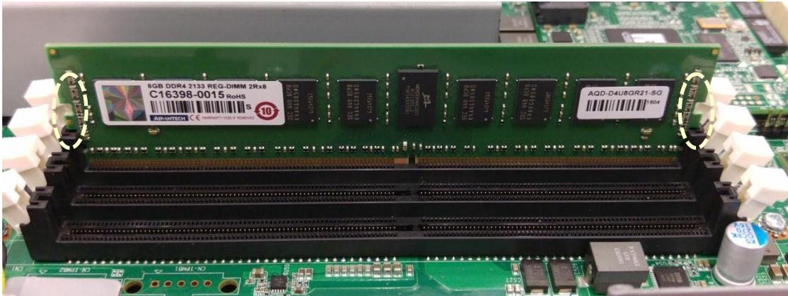
**Figure 65: DIMM insertion into slide rails**
