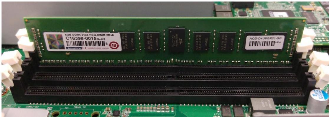
**Figure 66: Seating the DIMM in the socket**
