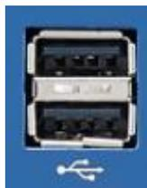
**Figure 71: Stacked USB Type A connector**
