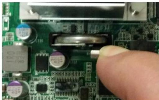
**Figure 67: Unlocking the battery**
