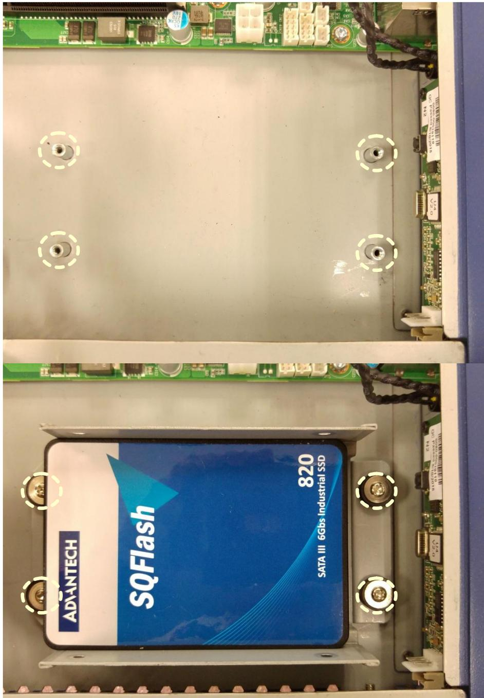
**Figure 55: Insertion of the carrier into the chassis**
