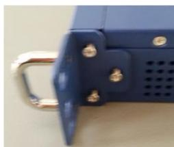
**Figure 2: Mounting ear screws inserted but not fastened yet**
