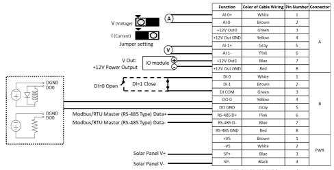
NOTE: PIN RS-485 GND is reserved to connect system and external ground.
