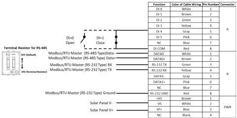
\*COM2 can be RS-485\_1 or RS-232, yet it cannot function at the same time with the both type
