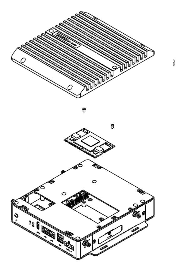
Step4: Put the Top Cover on and then lock 6 screws on top of it
