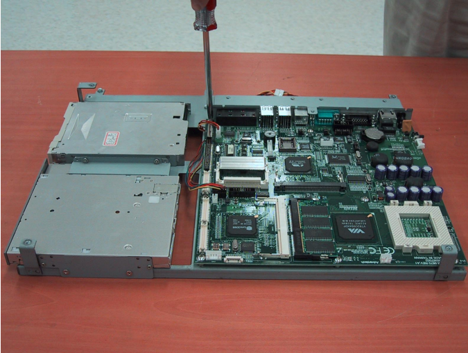
Figure B-8: Remove the CPU board
