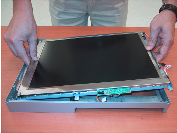
Figure B-6: Remove the rear cover
