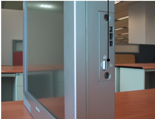
Figure 2-7: Power switch in open status
