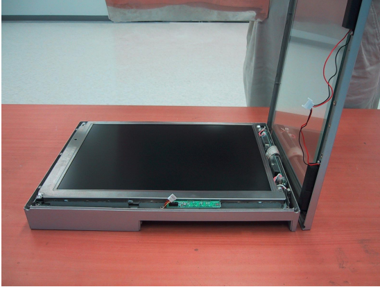
Figure B-4: Flip the front panel
