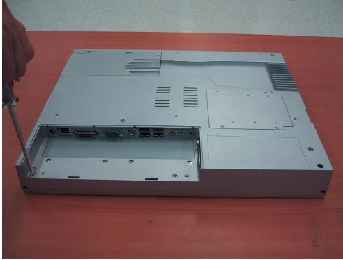
Figure B-2: Remove the screws on rear cover
