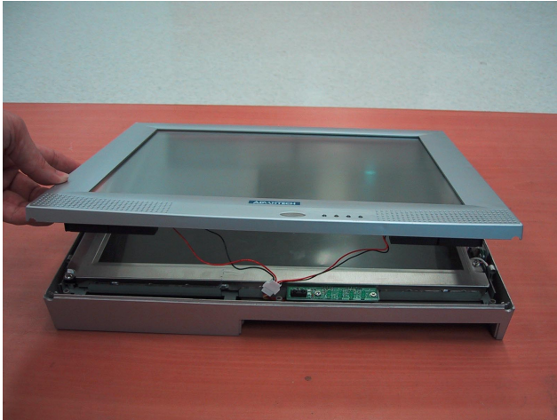
Figure B-3: Separate the front panel
