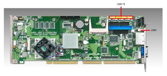
Figure 2.17 USB connector (USB1 to USB8)
