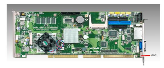
Figure 2.6 PS/2 Keyboard/Mouse Connector (KBMS1)
