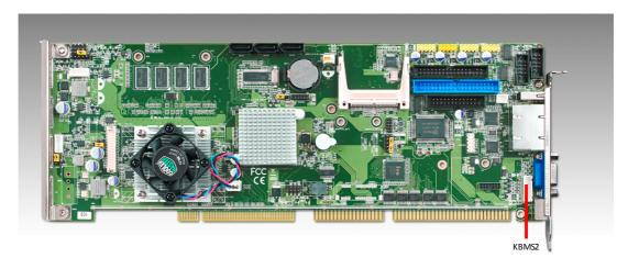
Figure 2.7 External Keyboard Connector (KBMS2)
