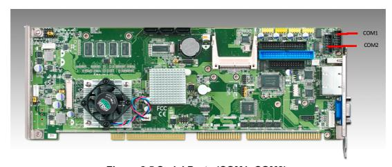
Figure 2.5 Serial Ports (COM1, COM2)
