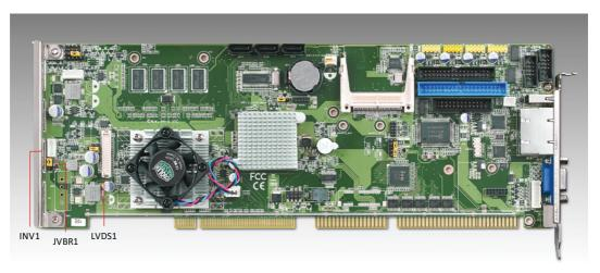
LVDS1 consists of a 40-pin connector which can support 18-bit single channel LVDS with resolution up 1366 x 768. The LCD inverter is connected to INV1 via a 5-pin connector to provide power to the LCD display. JVBR1 provides inverter voltage selection: close pins 1, 2 for 3.3V power input inverter; close pins 2, 3 for 5V power input inverter.
