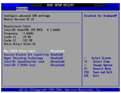
Figure 3.4 CPU Configuration Settings
