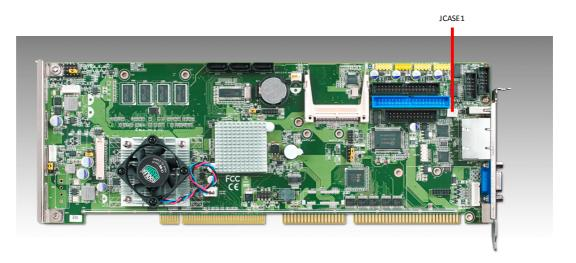
Figure 2.16 JCASE connector (JCASE1)
