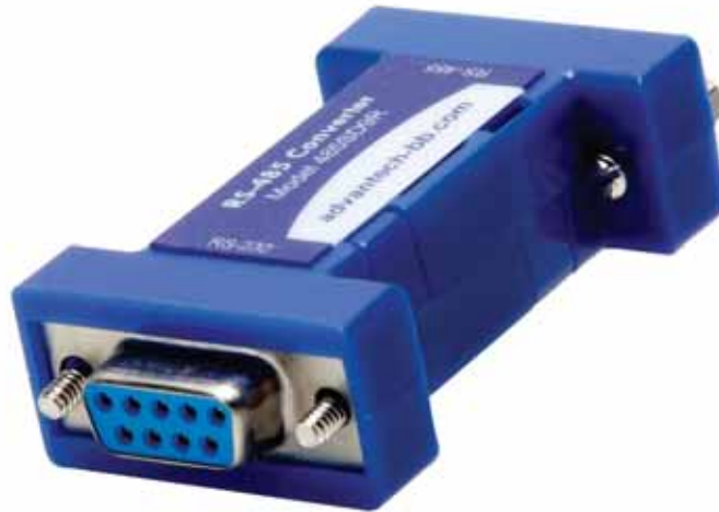
Figure 58: A Port Powered RS-232 to RS-485 Converter
