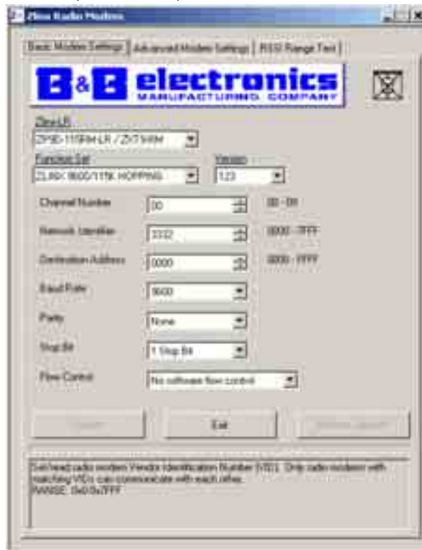
Figure 5-24 Basic Radio Modem Settings (ZXT9-RM)
