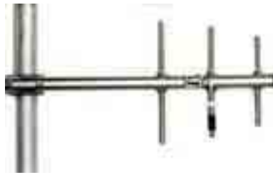
Figure 3-10 Representative Yagi Antenna Photograph
