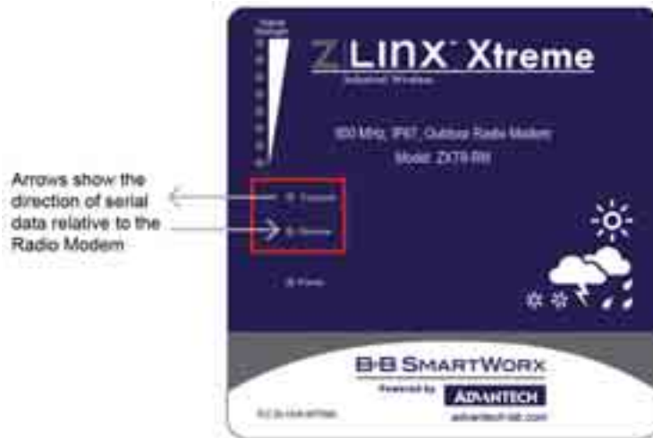
Figure 2-2 Transmit and Receive LEDs
