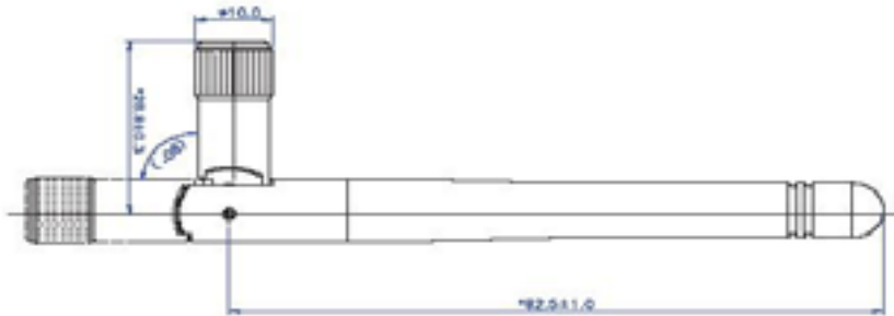
Figure 3-7 ZXT24-RM Supplied Antenna
