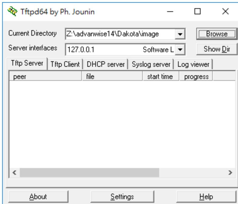
Step 6: Introduce 'tftp -r nand-ipq40xx-single.img -g 192.168.1.100' command to download firmware from NB/PC to WISE-3610. Finally, introduce 'sysupgrade -v nand-ipq40xx-single.img' to burn firmware into flash.
