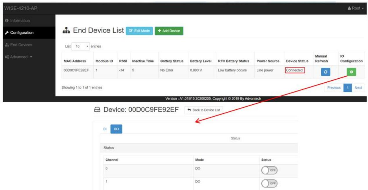
*Figure5. IO Configuration Page for Downlink Mode*
