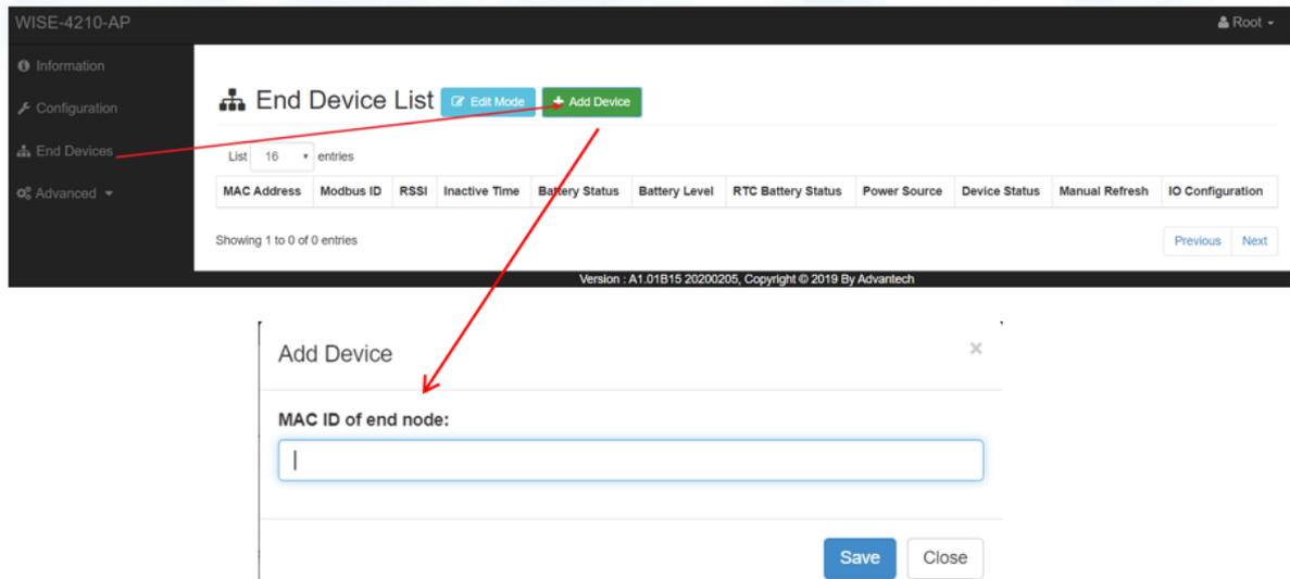
Figure3. Add Downlink Device into Connection List of WISE-4210 AP
