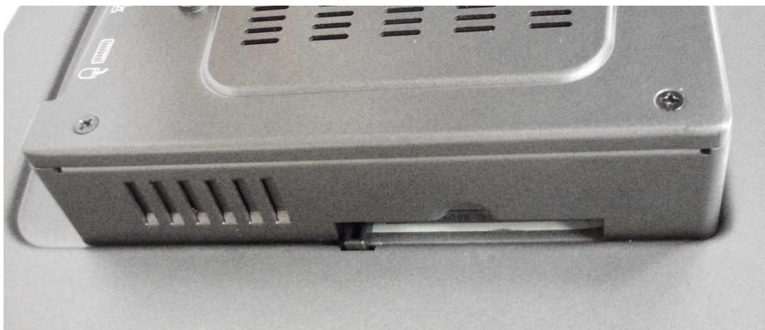
Figure 2.2 Install CompactFlash Memory Card
