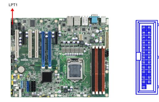
The parallel port is normally used to connect the motherboard to a printer. The ASMB-782 includes an onboard parallel port, accessed through a 25-pin flat-cable connector, LPT1.
