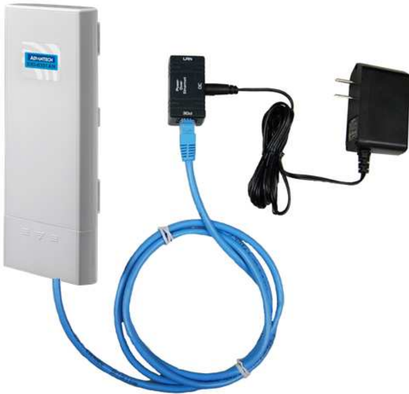
Figure 6 Plug the Ethernet cable to the RJ-45 jack of the injector
