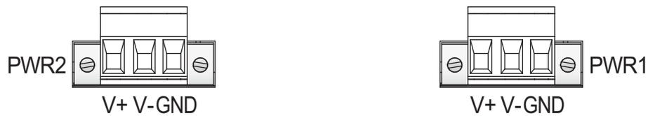
**Figure 2.14 Terminal Receptor: Power Input Contacts**
