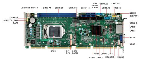
Figure 1: Board Layout: Jumper and Connector Locations
