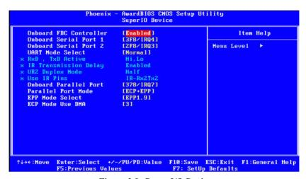
Figure 3.9: Super I/O Device
