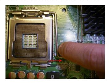
2. Align the triangular marking on the processor with the cut edge of the socket.
