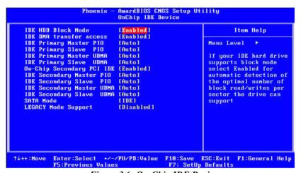
Figure 3.6: On-Chip IDE Device
