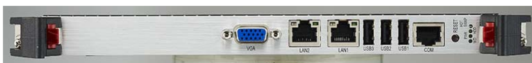
Figure 1.5 MIC-3397 4HP Front Panel Ports, Indicators and Buttons
