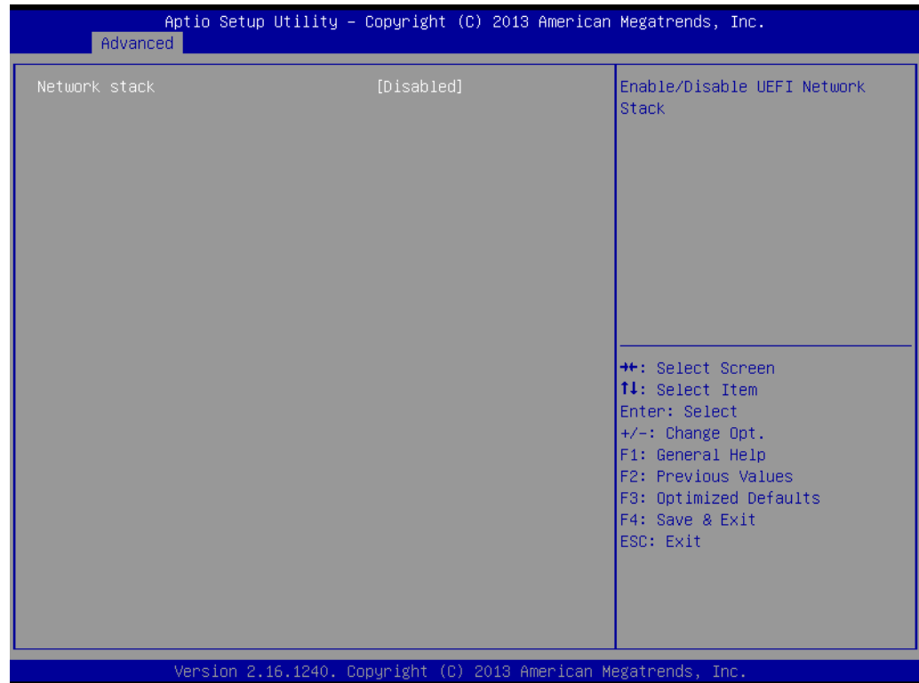
Figure 2.13 Network Stack configuration
