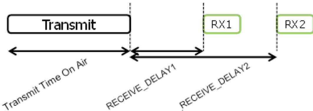
**Class A End-device receive slot timing.**
