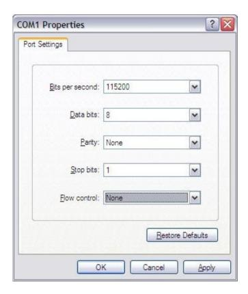
3. Insert power adapter to DC jack and power up the board. The Debug console log will be displayed on the terminal screen.
