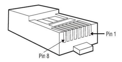
Figure A.1: RJ-45 Pin Assignments
