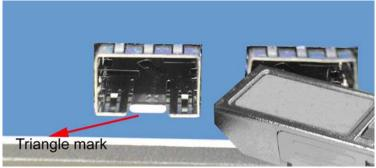
Figure 2.5-1 Transceiver to the SFP slot
