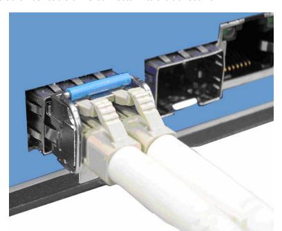
Figure 2.5-3 LC connector to the transceiver
