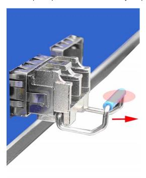
Figure 2.5-5 Pull out from the transceiver
