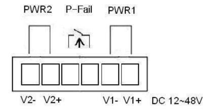
Figure 2.6-1 Pinouts of the Power Connector
