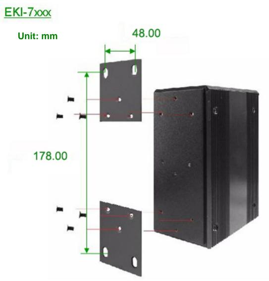
Figure 2.3-1 Combine the Metal Mounting Kit
