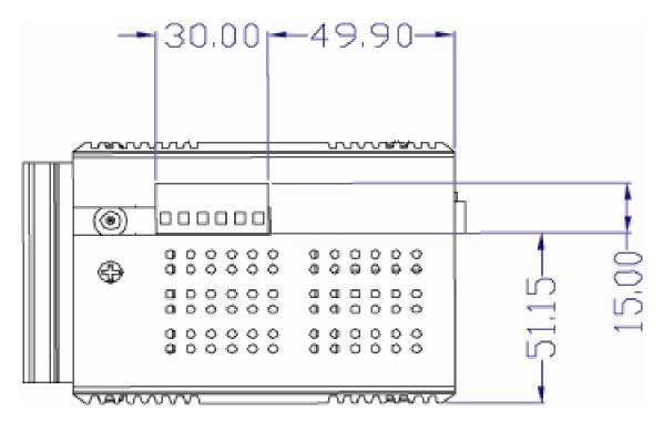
Figure 2.2-4 Top View of EKI-7758F
