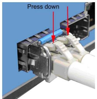
Figure 2.5-4 Remove LC connector
