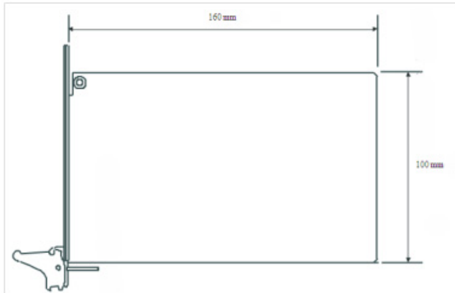
Figure 1.3 MIC-3327 Board Dimensions
