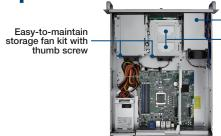
air duct for concentrated cooling air 2 x internal 2.5" HDD/ SSD bracket
