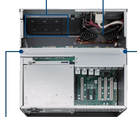
2 x 2.5" SSD install on the left and right sides
