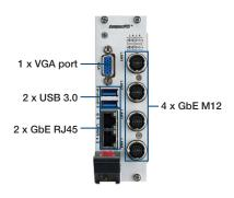
MIC-3332 4HP height with XTM-3 board IO functions
