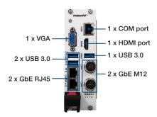
MIC-3332 8HP height with XTM-2 board IO functions
