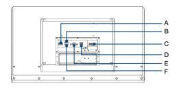
A. RX (RJ-45) B. DP C. 24V<sub>DC</sub>-Power Supply
