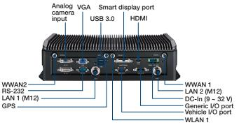
Note: WLAN 1 = WLAN main, WWAN 1 = WWAN main, WWAN 2 = WWAN auxiliary
